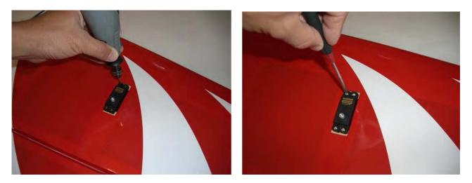
**step 4** Glue the fibreglass horn with medium CA into the aileron.
